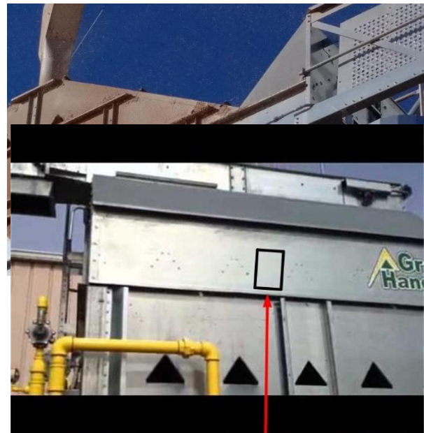
Install inlet (wet) sensor in vertical wall of roof section at least two ducts away from end wall and Figure 64 Sample inlet sensor installation on a Grain Handler dryer
