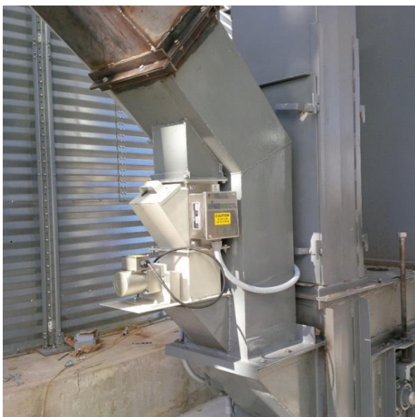
Figure 55 Example installations of bypass chute with rotary metering
